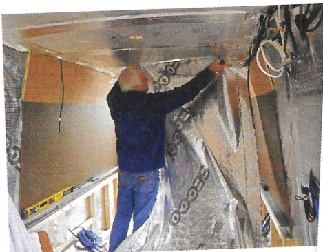
Putting in the insulation and wiring is the first job in a campervan conversion
